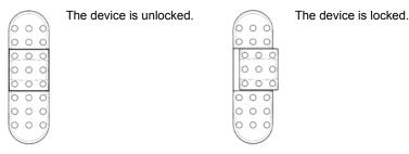
When you work with the DPM for the first time, insert the batteries and unlock the Lock/Hold switch. The device is now operational and you can insert the memory card.
